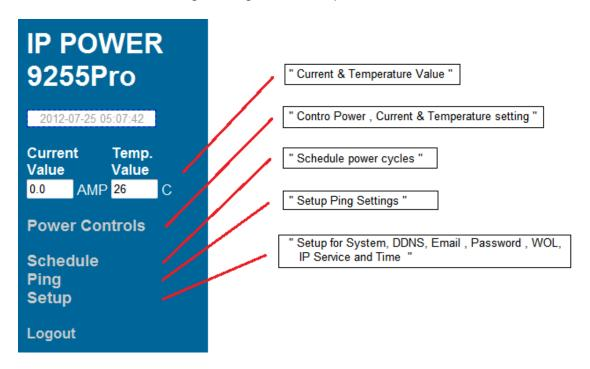
**Current & Temp. value :** show the consume current ampere and internal temperature at Celsius.
